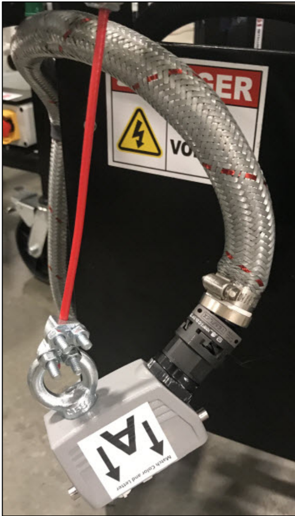
Figure 11 – Pigtail Cable Assembly
