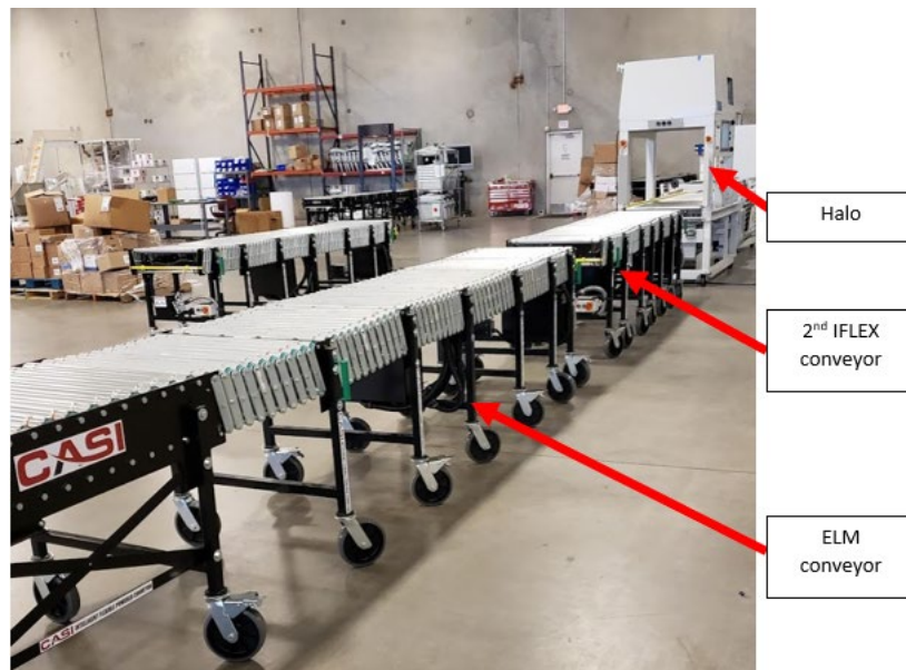
Figure 8 - Introduction of 2nd AFLEX Conveyor Between Halo and AFLEX with ELM Conveyor
