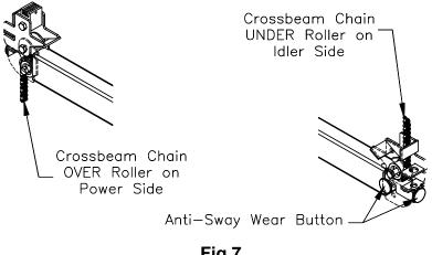
Fig 7 (Crossbeam Chain Arrangement)
