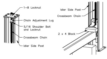
Fig 11 (Idler Side Column Installation)
