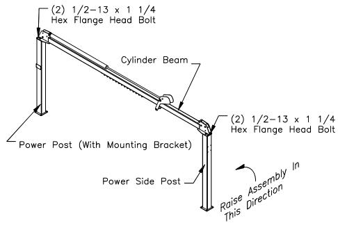
Fig 5 (Cylinder Beam / Power Side Post Assembly)
