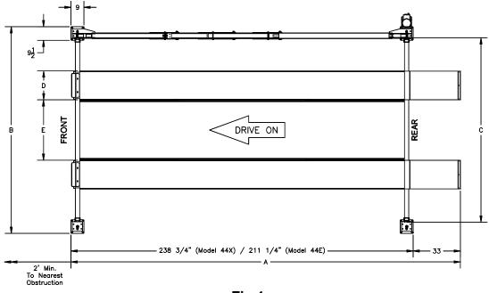
Fig 1 (Overall Lift Dimensions)
