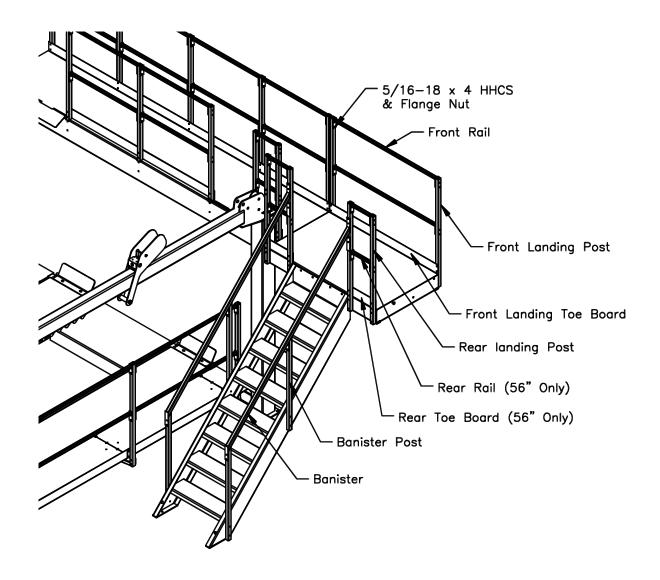
Fig 22 (Stair Railing Assembly)
