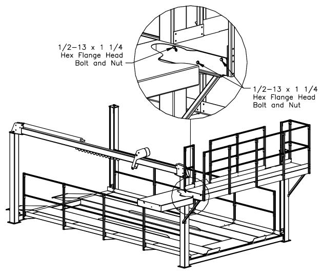
Fig 20 (Stair Landing) 7 Attach Stair Weld to the back of the Stair Landing using the ½-13 x 1 ¼ Hex Flange Bolts and Nuts provided. See Fig 21.
