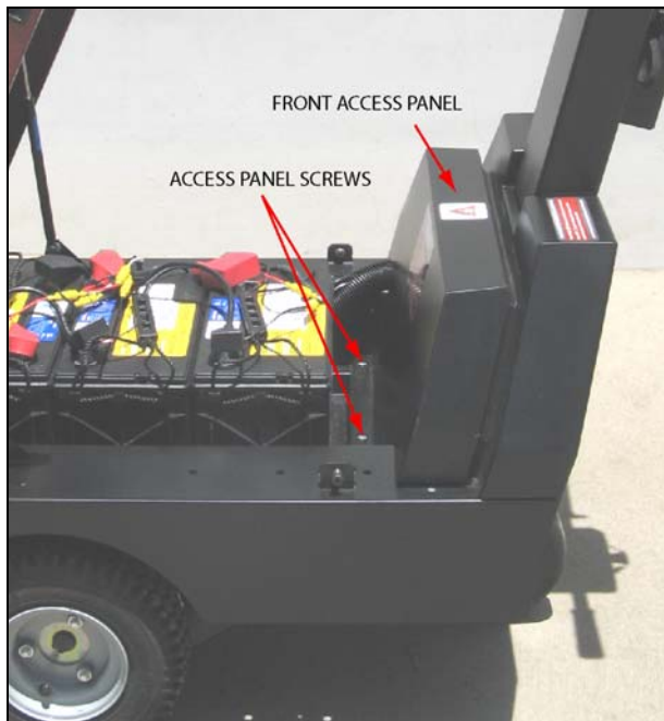
Front access panel screws
