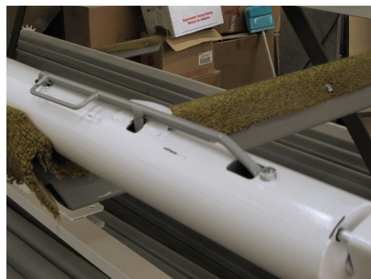
Reroller latch in unlocked position
