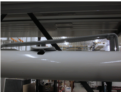
Reroller latch in the locked position Part # 111-0124
