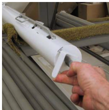
Reroller latch release lever. Pressing the lever releases the latches.
