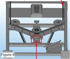
Load chain tightner adjustment bolt
