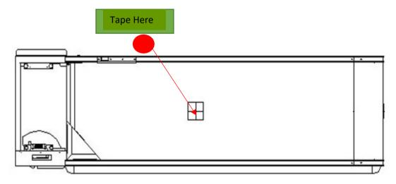
2. Run the belt, allowing the string to travel around the transport. When the taped end returns, stop the belt and cut the string where it meets the taped end.
