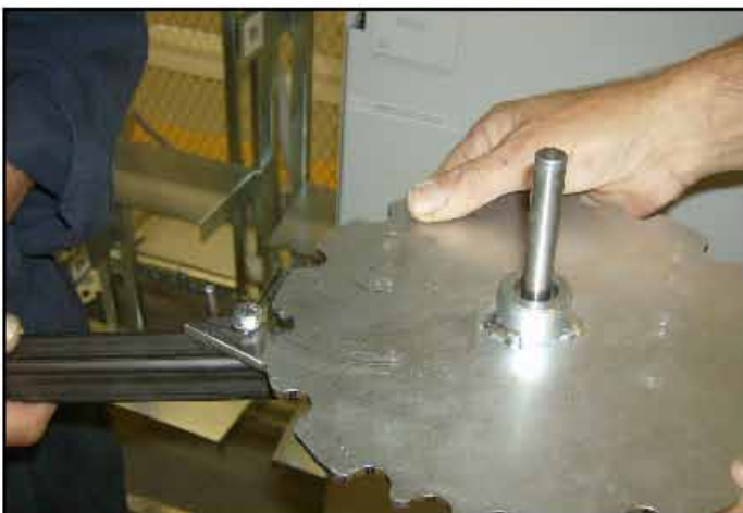
5. Place sprocket on the handle first ensuring it is holding the triangle in place.
