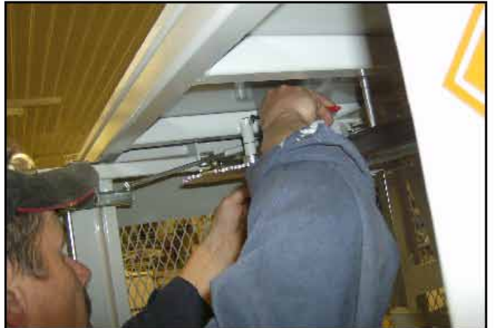
2. Remove snap ring from the top of the handle assembly in the cage.
