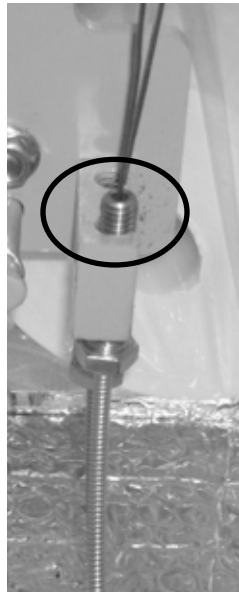
Fig. 17-D - Turn Bolt to Adjust
