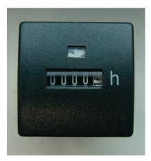
Vidir has installed an hour counter into our machine products. This counter will assist you to determine when Preventative Maintenance is to be scheduled (100 hours of machine use, or 12 months, whichever comes first).
