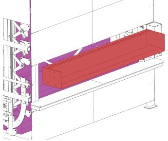
Rotate the carousel down by 1 position, and remove 1 additional shelf using steps A-D. Rotate the carousel down to allow access to the driveshaft.
