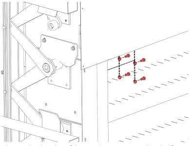
D) Zip-tie load arms together on both sides of the machine. Remove the shelf.
