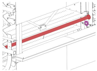
Level shelves up using Tape Measure, BEFORE tightening bolts down.
