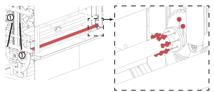
Using Ratchet straps, lift or lower to take pressure off of Drive Shaft Fastening bolts.
