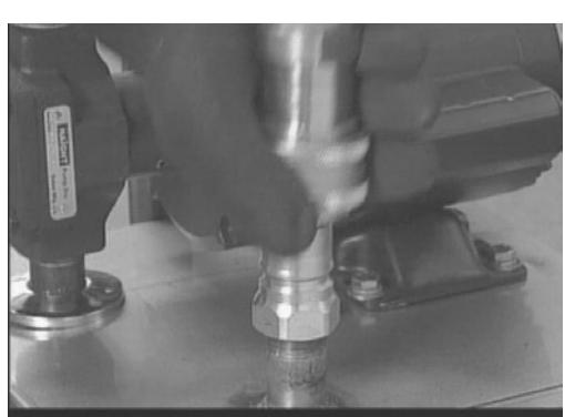
**15. Return the hose connection to the caddy and push the button on the panel for 5 seconds**
