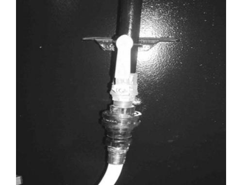
**9. Connect the hose to the Cleanstar tank and open the ball valve**
