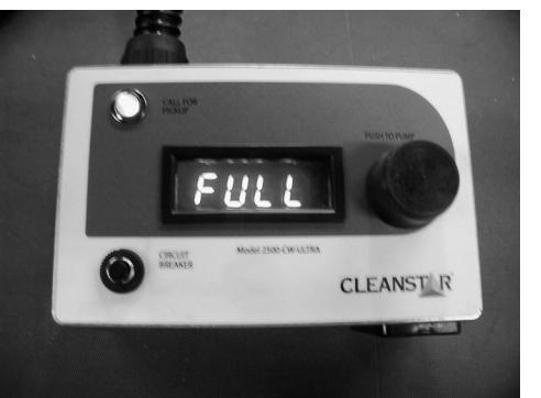
**20. When the indicator on the Control Panel reads Full, the tank is full and the pump will stop pumping**
