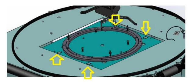
Install the clips/screws into the inner square holes (red arrows), as this will allow them clips to line up with the 18" bearings.
