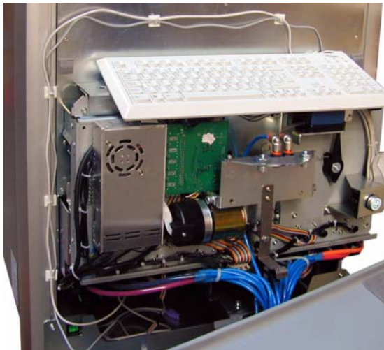
Figure 23: Fasten both the mouse cable and the keyboard cable to the mounts with cable ties.
