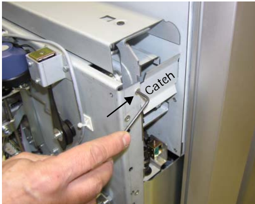
Figure 30: The catch that locks the dispensing module is fastened with one screw.
