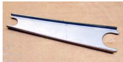
Figure 52: The special tool you need for replacing a pump and a canister.
