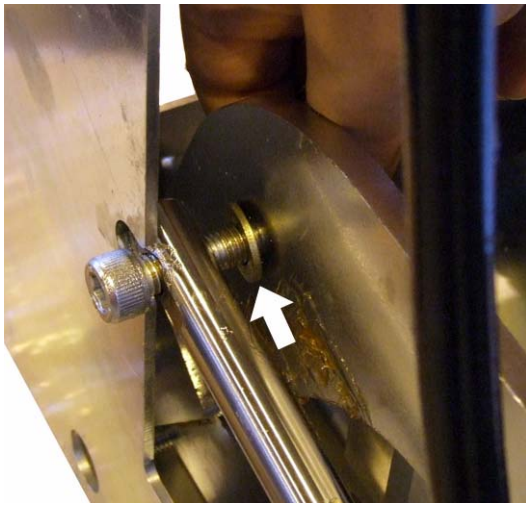
Figure 47: Fastening the cylinder rod to the can table assy.
