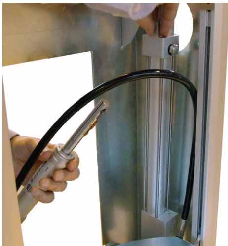
Figure 44: Install first the hydraulic unit's pump in position.
