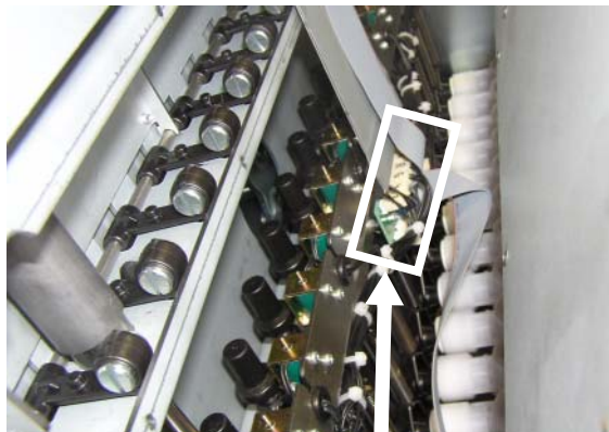
Figure 9: Interface board B is fastened to the solenoid rail assy behind the dispensing module.
