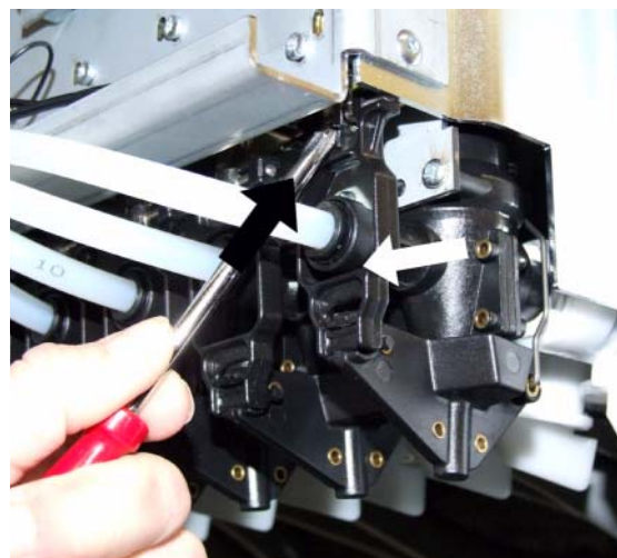
Figure 35: Push the plunger upwards until the draft bar touches the outlet of the pump (white arrow).
