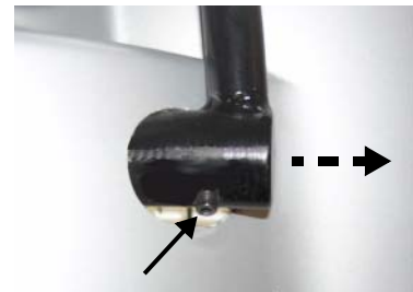
Figure 25: The puncher handle is attached to the crank with one locking nut.
