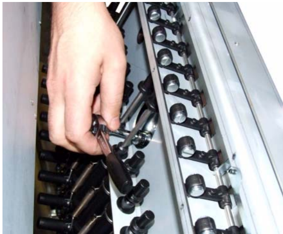
Figure 81: Use a socket wrench to remove the nut of the motor's driving crank.
