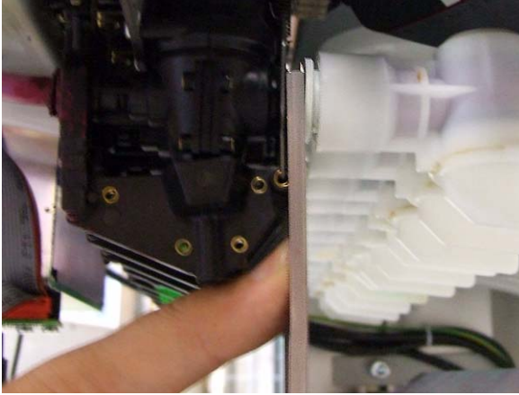
Figure 64: Place the tool between the pump and the sleeve and push away from the pump.
