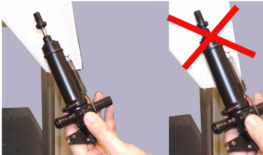
Figure 15: The piston of the pump must be lifted up a little, when the pumps are in the machine.
