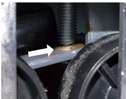
Figure 46: There is a washer on the lever at the bottom end of the connecting rod.
