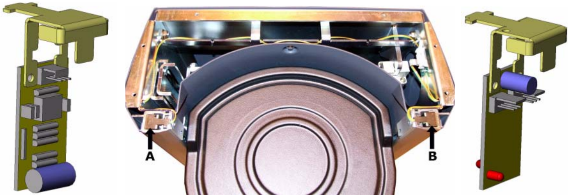
Figure 72: The can on can table -sensors, IR transmitter B and IR receiver A, are located in upper part of the can table assy.
