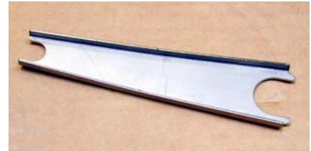
Figure 61: A special tool that is needed when you change a canister.
