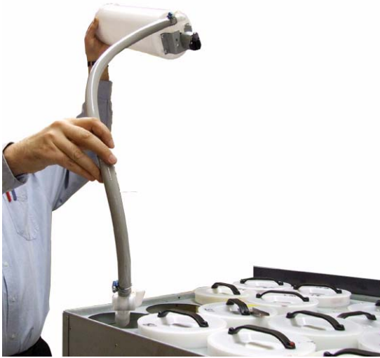
Figure 67: Thread the canister from above in position.
