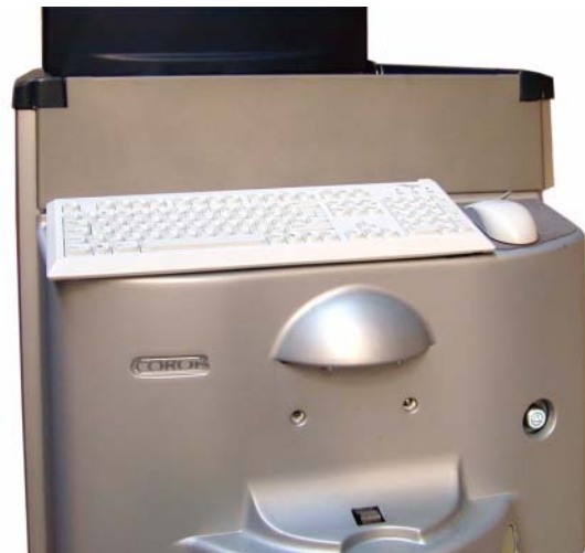
Figure 24: Put the front casing and panel back in place. Fasten the keyboard with stickers on top of the casing.
