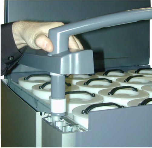
Figure 17: The monitor arm and corner frame are lifted up.
