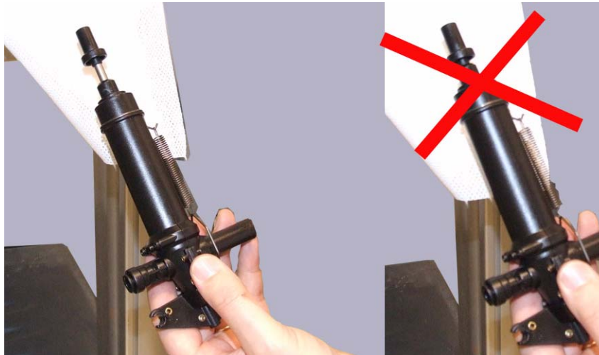
Figure 55: Install the pump so that the piston rod is lifted out a little.
