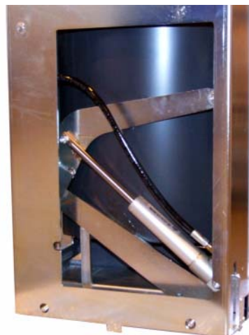
Figure 39: The hydraulic lift unit in position in the can table.
