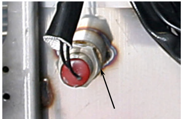
Place wrench here when removing and installing high-limit.
