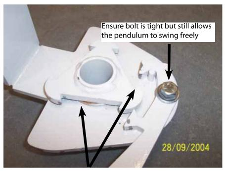
To eliminate squeaking apply a lightweight oil to the moving parts
