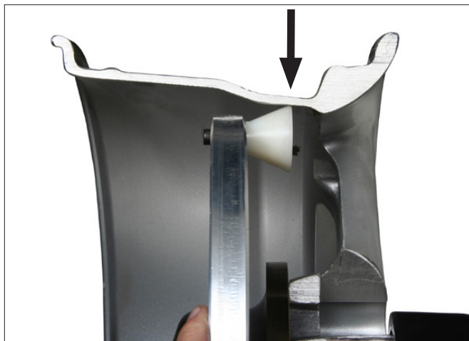
Figure 12 - Hidden Weight Location Viewed on a Cut Away Rim for Clarification.
