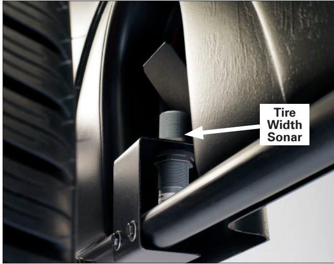
Figure 18 - Tire Width Sonar Located Inside Hood
