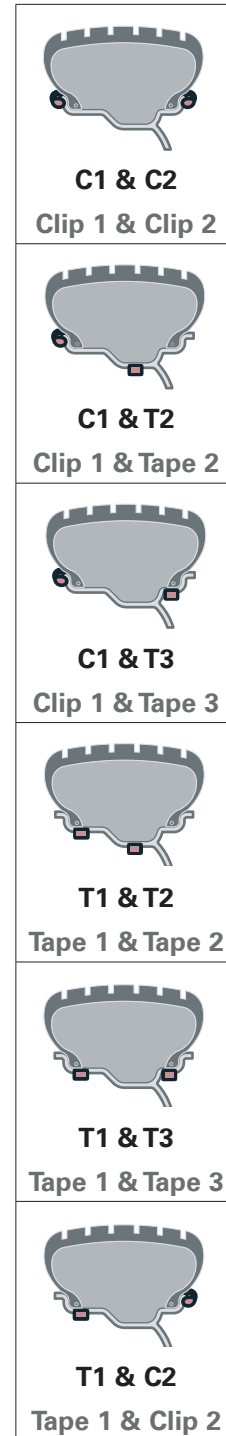
Figure 32 - Dynamic Balance Weight Locations
