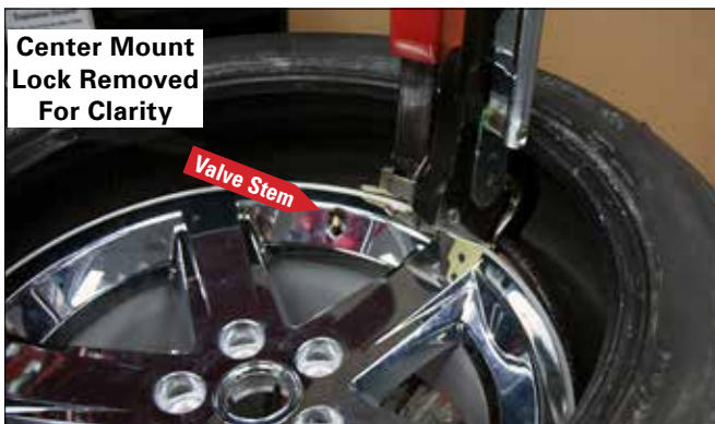
Figure 53 - Bead Lifter Tool Hooked Under Lower Tire Bead
