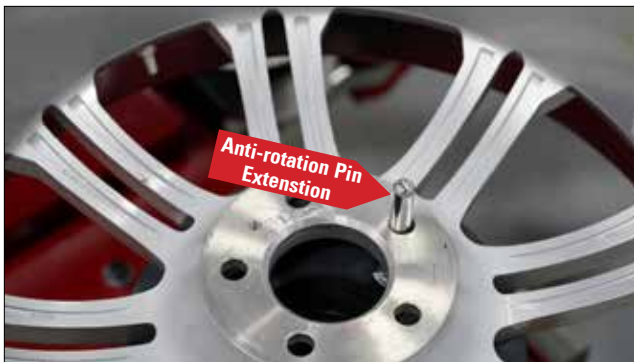
Figure 8c - Place Reverse Mount Tire/Wheel Assembly on Pedestal with Anti-Rotation Extension Pin in Lug Hole
