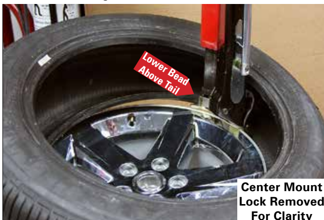
Figure 58 - Position Tire Against Bead Lifter Tool
