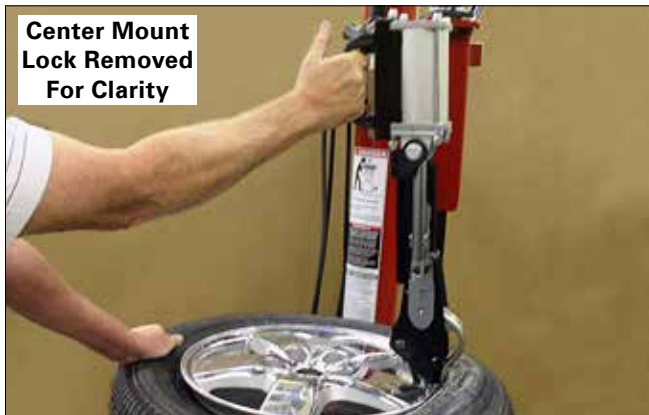
Figure 51 - Leverless Tool Hooked Under Tire Bead
