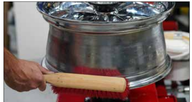
Figure 21 - Inspect and Clean the Wheel
