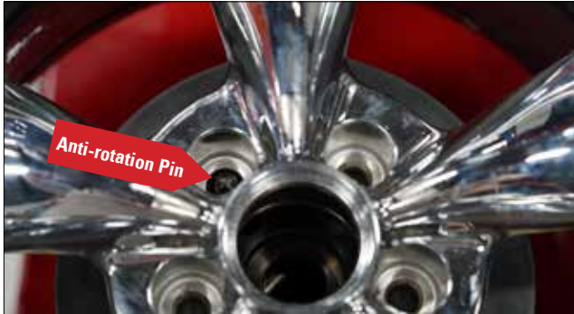
Figure 8a - Place Conventional Tire/Wheel Assembly on Pedestal with Anti-Rotation Pin in Lug Hole
