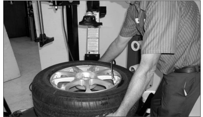
Figure 23 - Lift Tire Upwards for Bead Sealing
