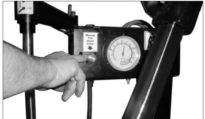
Figure 25 - Location of Manual Release Valve
