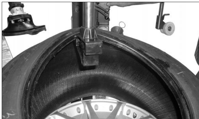
Figure 13 - Lift the Tire for Lower Bead Removal
