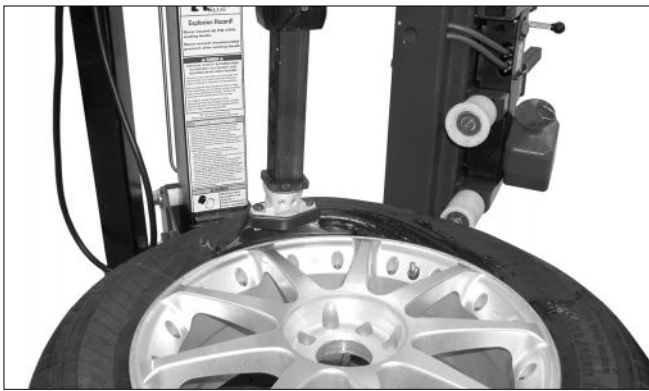
Figure 12 - Demount Upper Bead
