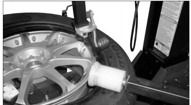
Figure 21A - Use Power Roller To Hold Tire In Rim Drop Center
