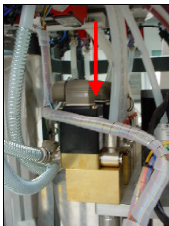
picture 6-10 Exchanging the electro valve
