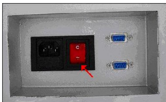
picture 5-8 Main switch
