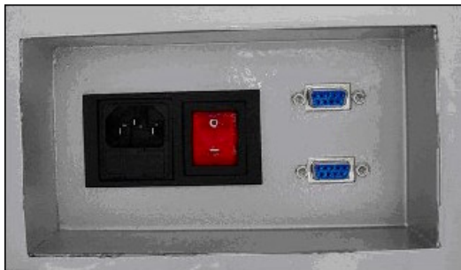
picture 5-6 Insert power(01) and serial cable (02)
