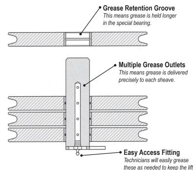
Solving the needs of all lift industry distributors remains one of SVI's top specialties. In this case, several of the industry's most respected distributors asked us to develop greaseable sheaves and sheave pins for 4-post lifts to reduce the frequency with which standard sheaves and pins are replaced.
