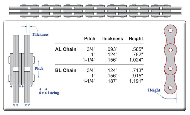
SVI supplies chains in four convenient lengths; 10, 25, 50, and 100ft. Connecting links are also available for use in joining various lengths of the same size chain together.
